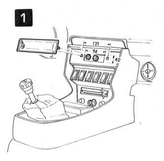
Provision is made in this model for the installation of the radio and speakers.
